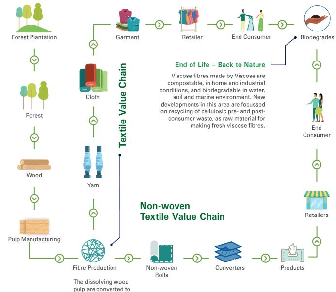
The dissolving wood pulp are converted to cellulosic fibres such as viscose, modal, lyocell and non-woven.
